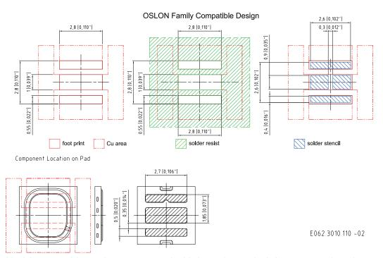
For superior solder joint connectivity results we recommend soldering under standard nitrogen atmosphere. In case the PCB layout of the application is intended to be used with other OSLON derivates or in future developed OSLON derivates, the heat sink must not be electrically connected to anode or cathode solder pad because of possible chip inverted polarity. Package not suitable for ultra sonic cleaning.
